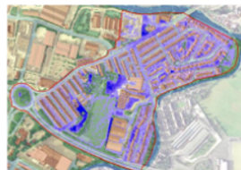
CADDIES 2D surface flood model output example: maximum inundation values in an urban area
